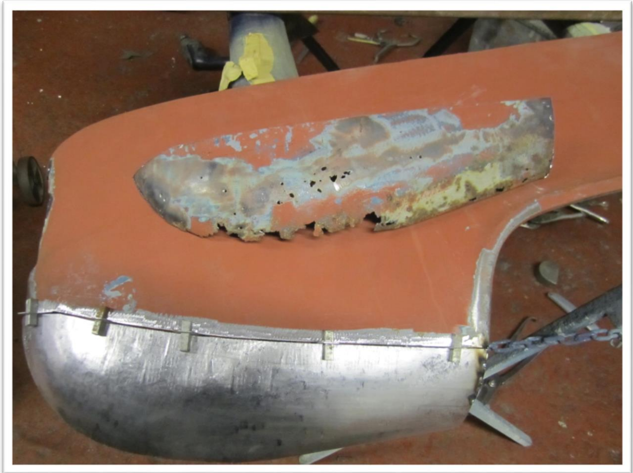
Figure 5 – Lower Rear Wing Professional Repair
