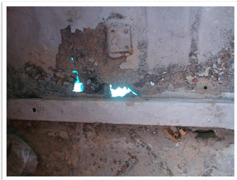
Figure 2 – Severe Rear Floorpan Rot
