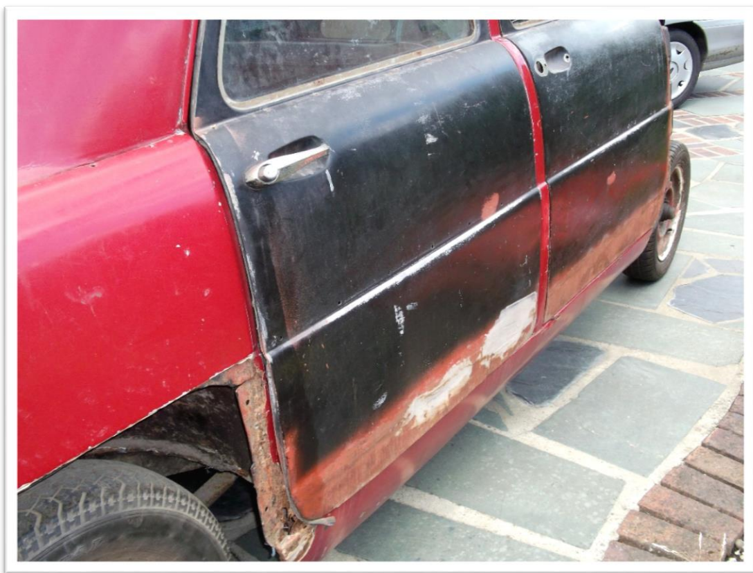
Figure 3 – Typical Door Rot and Repairs
